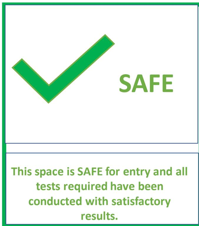
A space which is safe to enter and all necessary measures to ensure the safety as required by the ship's SMS have been implemented ensuring the safety of those entering it
