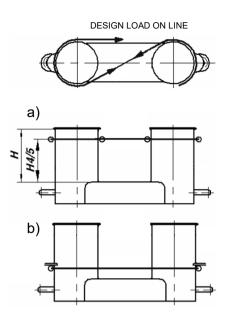
4.5.3 Under the design load conditions, as specified in 4.3, the allowable normal stress should be taken as 100% and the allowable shearing stress as 60% of the specified yield point for the material used. Normal stress is the sum of bending stress and axial stress with the corresponding shearing stress acting perpendicular to the normal stress, no stress concentration factors being taken into account.
