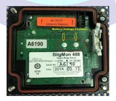
The newer model BilgMon 488 is equipped with a replaceable battery shown on the right below the yellow arrow. As a result, when the battery weakens the unit display will read "Batterylow: 0.5V Replace battery." The battery can then be safely removed because it utilizes a capacitor that ensures enough energy to maintain the stored data for several hours. Click here for the applicable manual.
